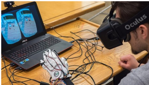
Fig. 5. Virtual Reality glove for haptic exploration. Credits: Pennstatenews.
